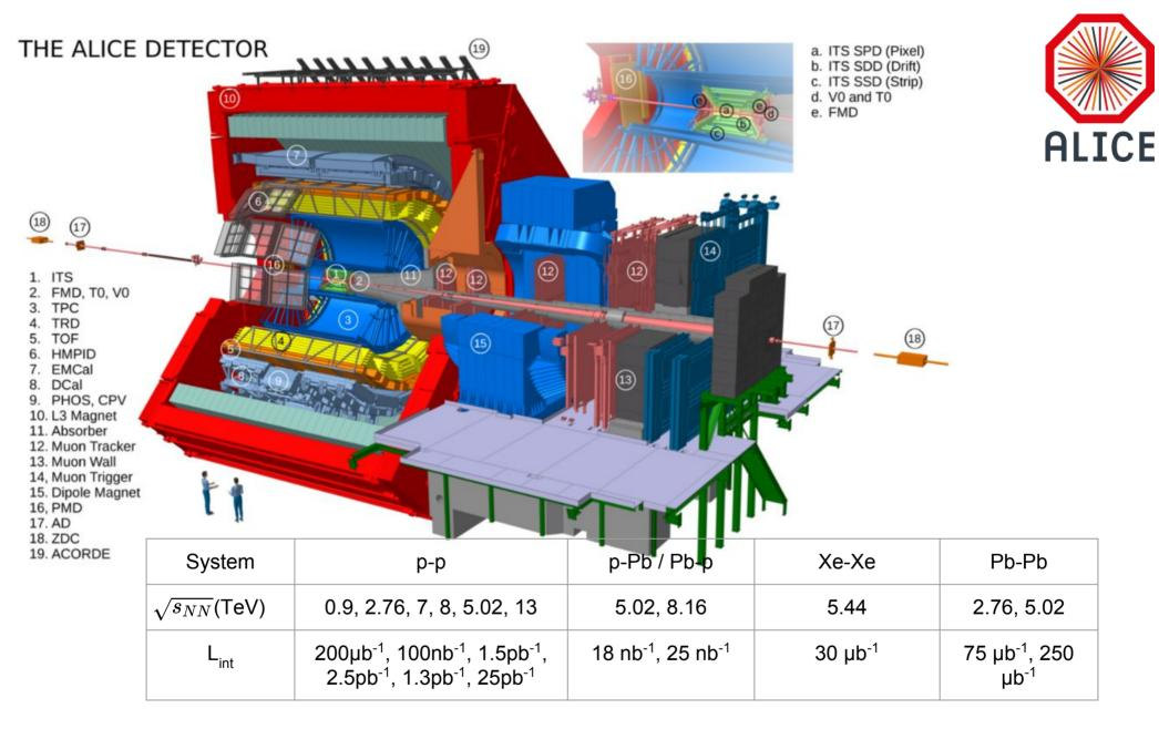
Dedicated detector to exploit the unique physics potential of nucleus-nucleus collisions at LHC Study the physics of strongly interacting matter at the highest energy densities reached so far in laboratory Comprehensive studies of hadrons, electrons, muons and photons to understand and describe QGP formation in heavy ion collisions
