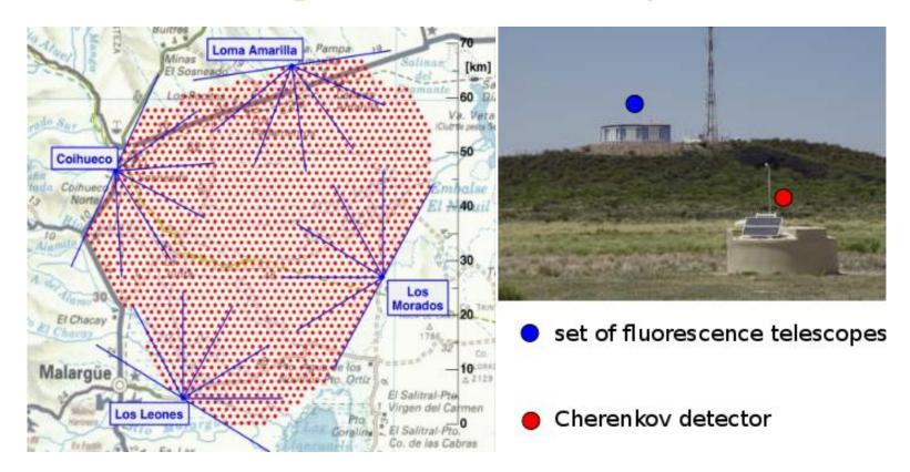
Surface Detector (SD) array: 1600 water-Cherenkov detectors spread over an area of 3000 km<sup>2</sup> (a bit larger than the country of Luxemburg)
