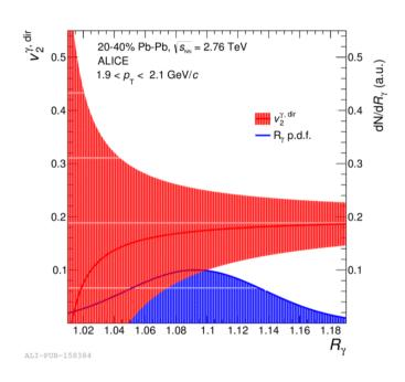
$$v_2^{\gamma, ext{dir}} = rac{R_\gamma \cdot v_2^{\gamma, ext{inc}} - v_2^{\gamma, ext{dec}}}{R_\gamma - 1}$$
