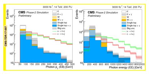
combination of this distributions is used in statistical analysis for limit settings with the asymptotic  $CL_S$  method.
